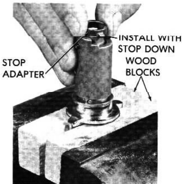
Figure 00-6 Installing Stop Adapter on Lock Cylinder
