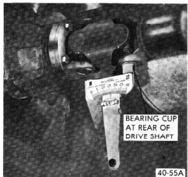
Figure 40-55A - Measuring Angle at Rear of Propeller Shaft
