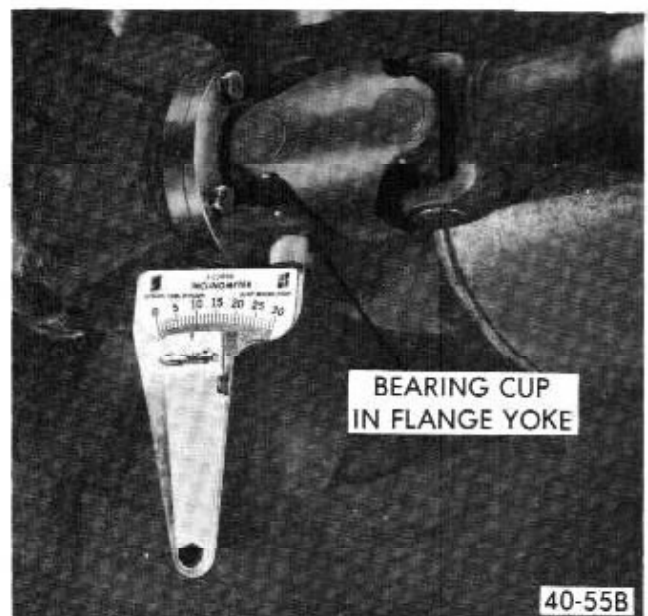
Figure 40-55B - Measuring Angle at Rear of Propeller Shaft
