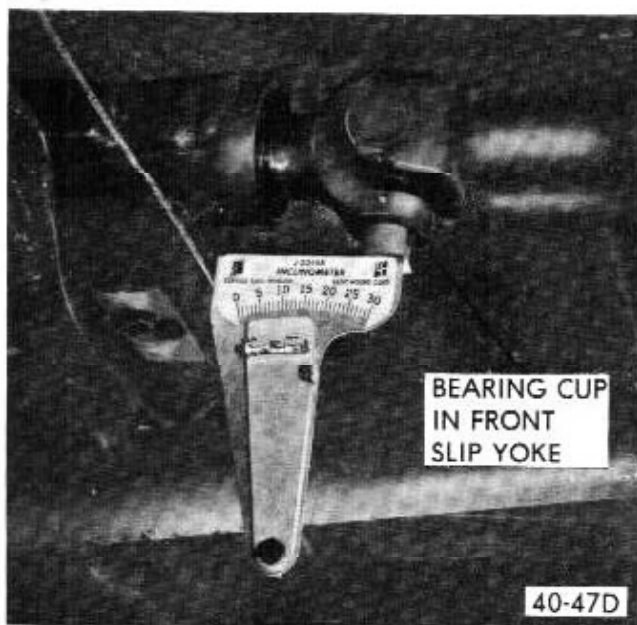
Figure 40-55 Measuring Angle at Front of Propeller Shaft
