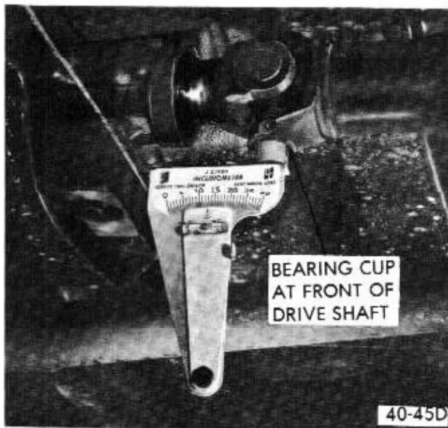
Figure 40-54 Measuring Angle at Front or Propeller Shaft
