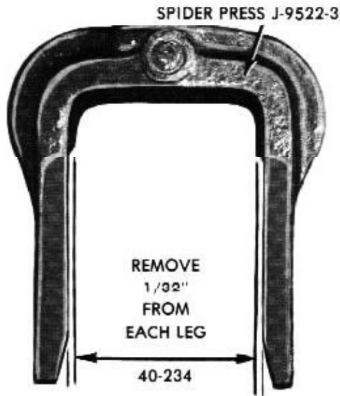
Figure 40-65 Spider Press Leg Rework
