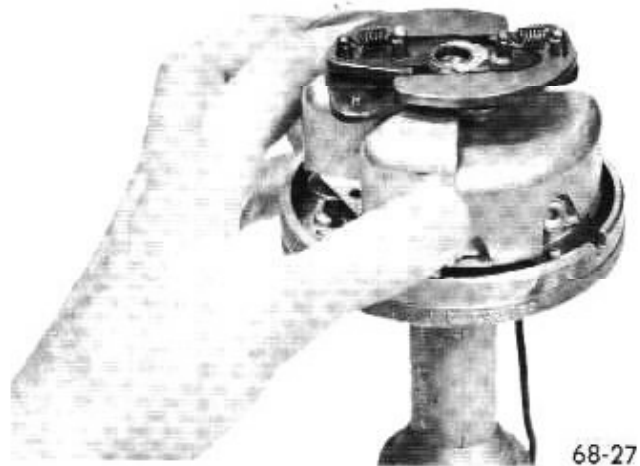
Figure 68-27 Installing Ignition Point Shield
