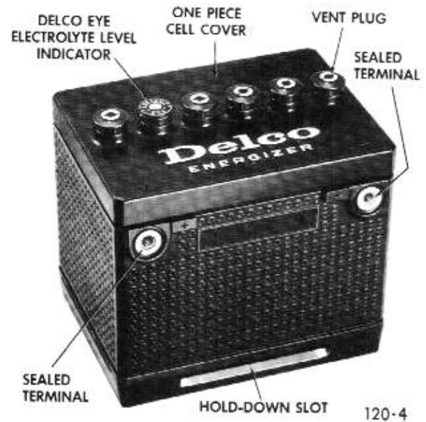
Figure 120-4 Side Terminal Battery - 45-46-48-49000 Series
