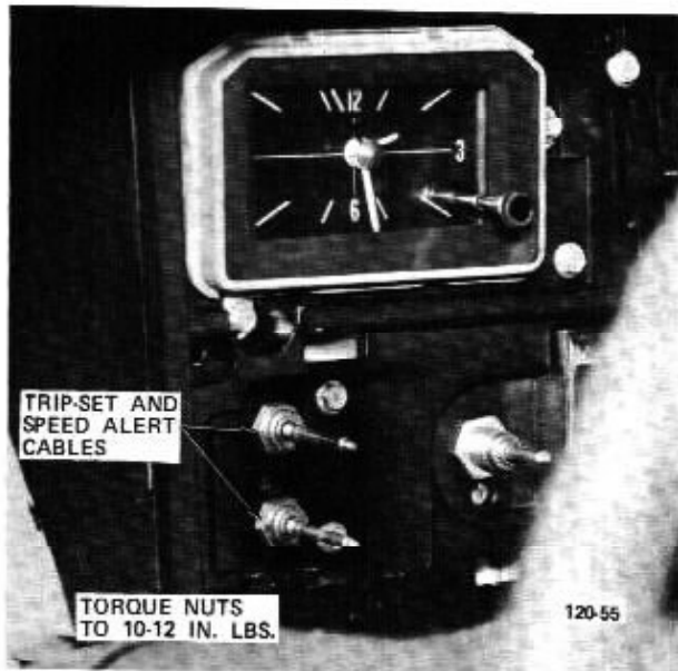
Figure 120-55 Speed-Alert and Trip-Set Cables
