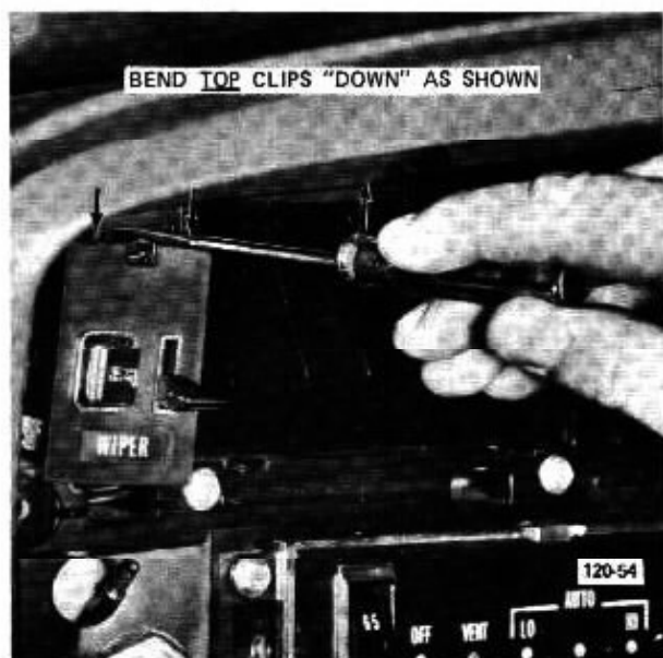
Figure 120-54 Removing Windshield Wiper Switch
